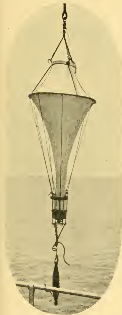
FIG. 19.—HENSEN'S LARGE PLANKTON NET. (From Chun.)
